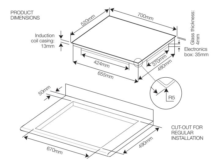
Glass thickness: 4mm Induction coil casing: 15mm Electronics box: 35mm Overall height: 52mm
